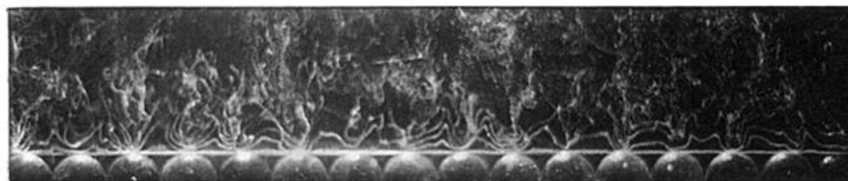
Figure 17. Near wall flow structure visualized by hydrogen bubble tracers generated on transverse wire parallel to the bed. Bed roughness conditions and wire distance from top of roughness, y_1 , follows: (a) smooth: y_1 = 1 mm; (b) k = 1.15 mm, y_1 = 1 mm; (c) k = 6 mm, y_1 = 3 mm; (d) k = 12 mm, y_1 = 3.5 mm; (e) k = 12 mm, y_1 = 0.55 mm.
